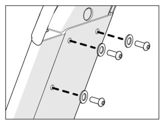
Figure 13: Fairing assembly attachment
