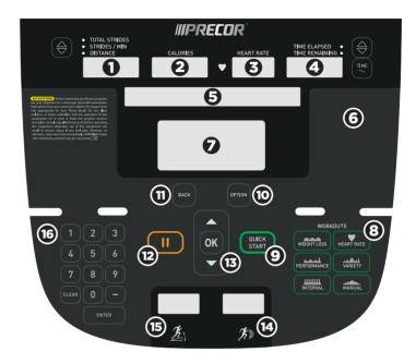
Figure 4: P30 console keys
