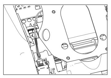
Figure 24: Connecting the heart rate cable
