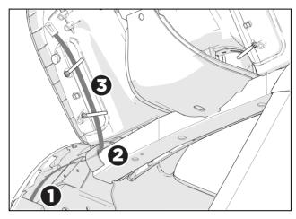
Figure 11: Base unit data cable positioning
