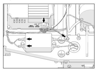
Figure 6: Removal of existing power harness
