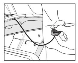
Figure 37: Attaching the safety clip
