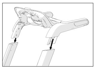
Figure 10: Fairing position in upright supports
