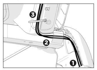
Figure 12: Console cable assembly positioning
