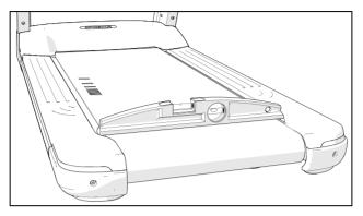
Figure 19: Bubble level placement on running belt
