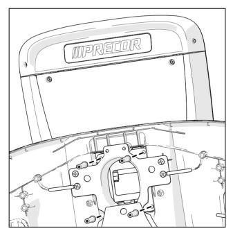
Figure 29: Securing the console
