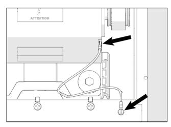
Figure 14: Electrical bleed line connection points
