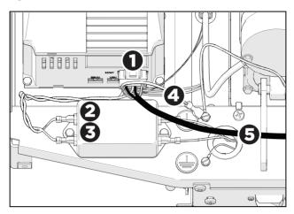
Figure 7: P80 power harness connection points
