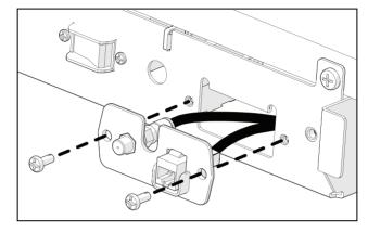
Figure 9: Accessory jack panel installation
