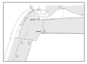
Figure 31: Access panel attachment
