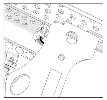
Figure 25: Connecting the power cable
