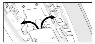
Figure 27: Cable routing from the mount into the console
