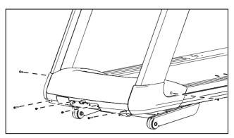
Figure 18: Hood installation and attachment
