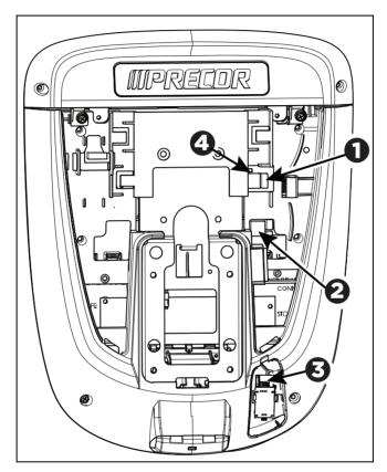
Figure 28: Cable connections, P30 and P10 consoles
