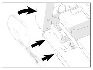
Figure 16: Corner cover positioning
