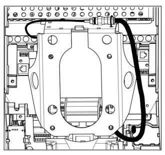
Figure 22: Connecting the television cable
