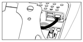
Figure 23: Connecting the Ethernet and base unit data cables
