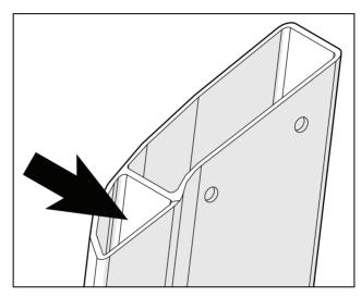
Figure 3: Cable channel location
